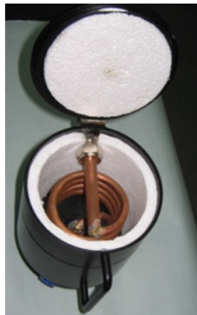
Condenser inside view
