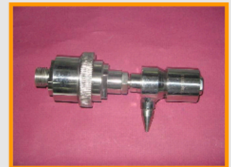
PM 2.5 Cyclone-Filter Holder
