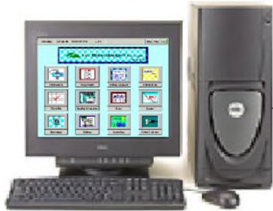
Station Manager CEM Data Logger PC
