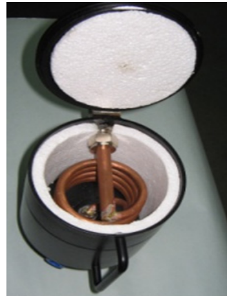
Condenser inside view
