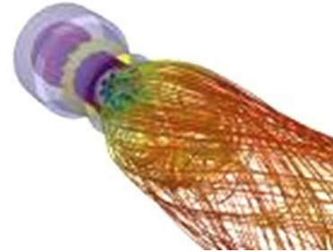
Figure 2- CFD depiction of the turbulent mixing of fuel and air through a burner.
