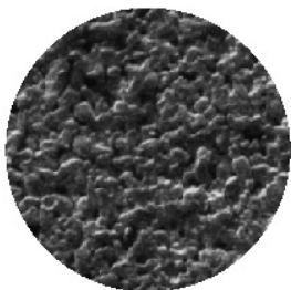
0.5µm (shown here, x100) is the recommended micrometer grade for filter applications. also provides filters with all-metal media in 0.2µm, 2µm, 5µm and 10µm.
