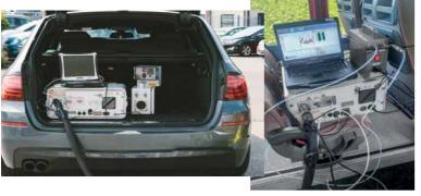
Gas Chromatography (GC-TCD FID PID MS ECD) analyzers
